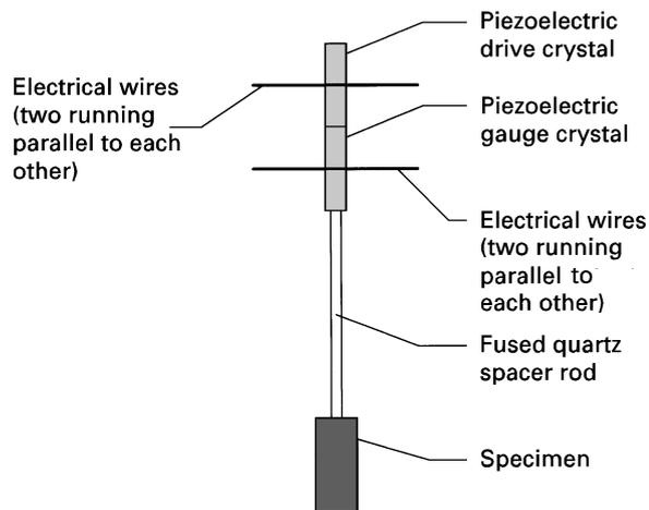
Figure 2 Schematic drawing of the piezoelectric ultrasonic composite oscillator technique.
