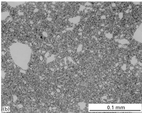
Figure 1 Microstructures of HIPed NiAl-AIN composites, containing (a) 1% AlN, and (b) 30% AlN.
