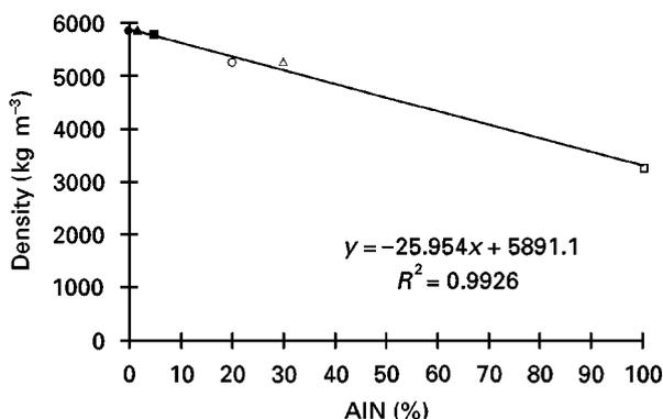
Figure 4 Density versus percentage of AlN for NiAl–AlN compounds, with the datum for the 10% AlN specimen removed, ( $\bullet$ ) 0% AlN, ( $\blacktriangle$ ) 1% AlN, ( $\blacksquare$ ) 5% AlN, ( $\circ$ ) 20% AlN, ( $\Delta$ ) 30% AlN, ( $\square$ ) 100% AlN.
